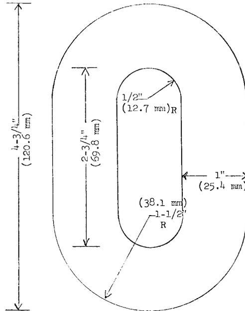
FIG. 4 Test Specimen
