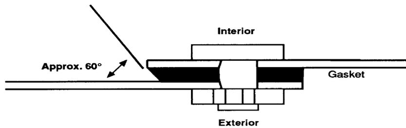
FIGURE 1- Undercutting gaskets
